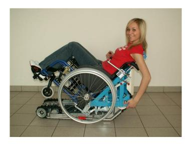
The wheelchair driver can now move on horizontal areas, either for carrying the **Stairmax** from one location to another (e.g.: from the car to the stairs or from the stairs to a parking location) or to turn the **Stairmax** on landings between two stair flights.
