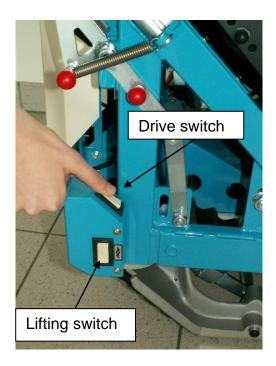
The lifting and drive rocker switches can be operated on both sides of the vehicle.
