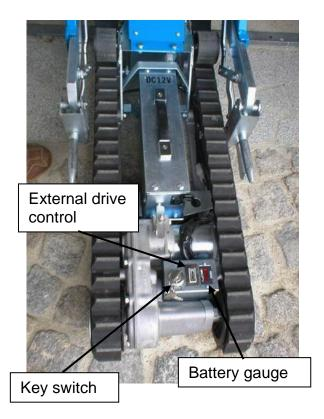
Key switch for ON/OFF and external drive control allow external operation
