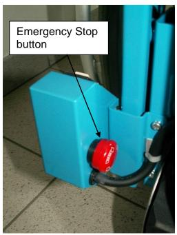
Emergency Stop buttons are also located on both sides behind the rocker switches. When pushed, they disconnect the electricity supply to the motor.
