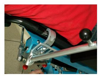
After tilting backwards and fixing of the wheelchair with the locking brackets the wheelchair driver always has to make sure that both sides of the wheelchair backrest are securely clutched by both locking brackets (on both sides).
