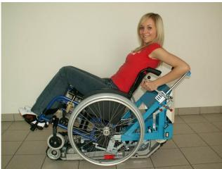
When attaching the wheelchair to the **Stairmax** the adaptation pipes have to run over the adaptation holder profiles. Now the wheelchair can be tilted backwards. When tilting backwards, the **Stairmax** is automatically attached to the wheelchair by locking of the adaptation hooks.
