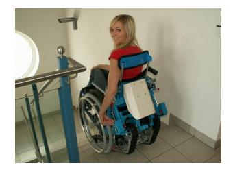
The wheelchair driver has to establish his individual tilting point by slowly approaching the first upper step. In general the tilting point is reached when the wheelchair axis passed the edge of the first step. Here the *Stairmax* should be stopped and then it should be tilted by shortly holding on to the handrail and pushing the *Stairmax* forward.
