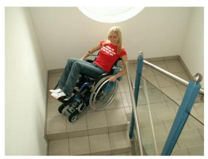
After reaching landing the between flights two the Stairmax has to be changed from Position 2 to Position 1 to allow for horizontal driving. To facilitate the turning on landings between stair flights Stairmax should drive upstairs on the inside of the stair as far as possible.
