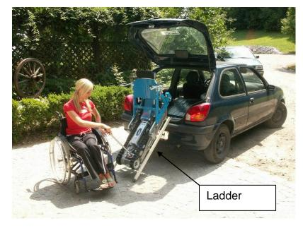
The same ladder can be used to move the **Stairmax** in and out of a car and enables for the easy transport from one location to another.
