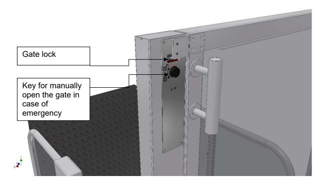
In case the door lock does not unlock electrically, it is possible to use the key to manually open the door lock and open the gate.
