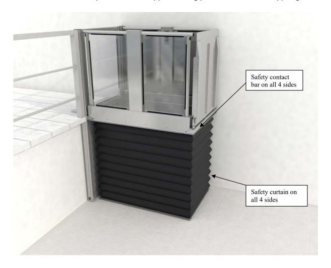
The platform is equipped with a safety curtain, protecting the lifting mechanism on all 4 sides. Furthermore the is a safety contact bar on the side of the upper platform floor that stops the platform in case of an obstacle being squezzed under the platform when the platform is lowering.
